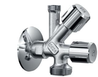
Combined angle valve 150252800 • Washmachine/washingmachine connection - 3/4" • Washbasin mixer connection - 3/8" • Wall connection - 1/2" • Adjustable, removable headpart • With tube connection
